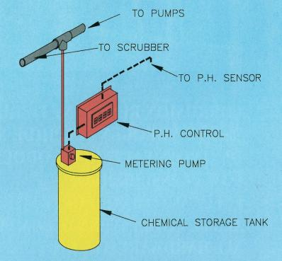
FOR APPLICATIONS ONLY REQUIRING THE NEUTRALIZATION OF ACID GASES IT IS POSSIBLE TO USE A SINGLE PH CONTROL SYSTEM, AS SHOWN ABOVE. SCRUBBER SIZES WILL VARY.
